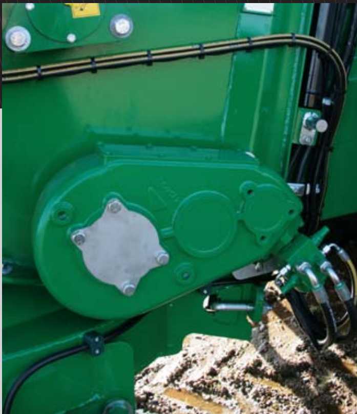
Stronger floor chain gearbox with a larger oil pump.
