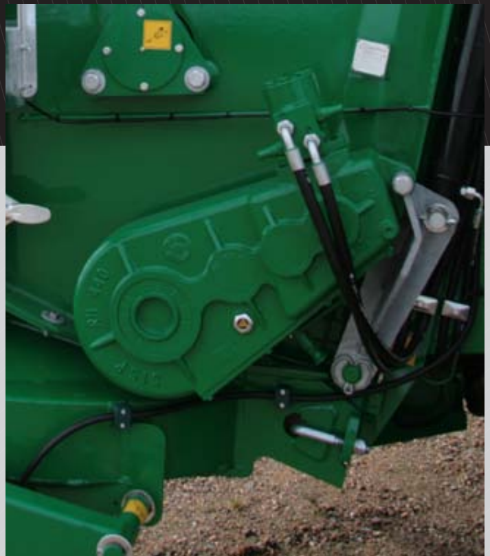
A two-speed gearbox can now be selected as an optional extra for the FLEX spreader.
