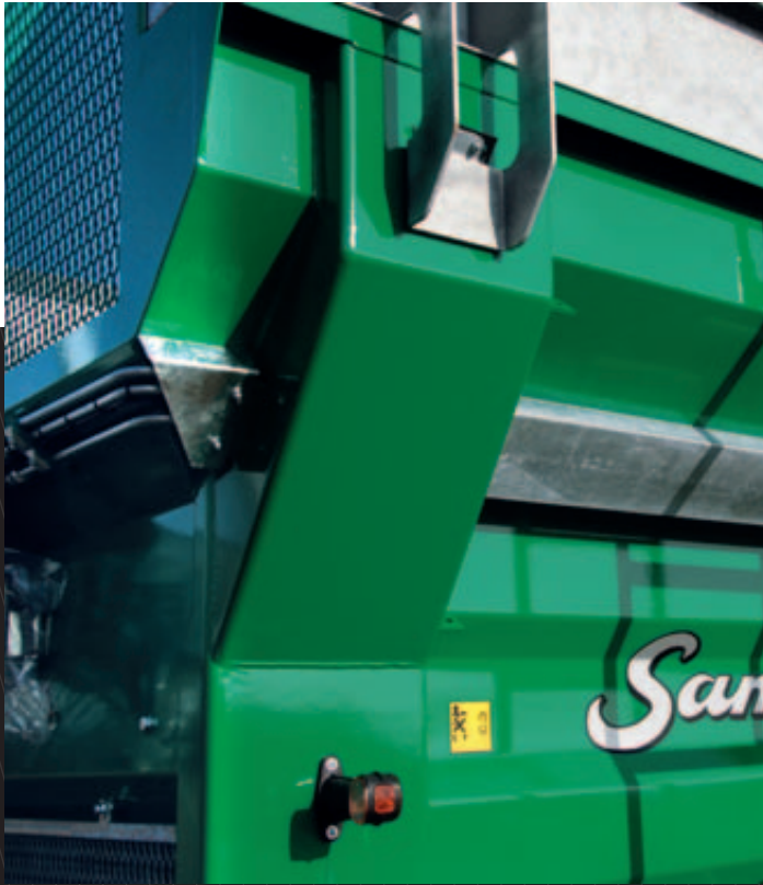
Hydraulics, hoses and cables are protected behind a bolted-on guard.
